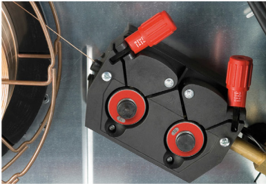
Quality wire feeder with 4 rollers.
