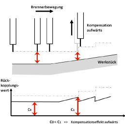
**Figure 6**: Principle of the evaluation of the "conventional" seam tracking signal for vertical guidance, image source: FANUC [4]
