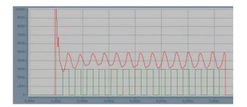
**Figure 9**: Recording of an oscillating, currentcontrolled impulse welding process on an angled sheet. Image source: User
