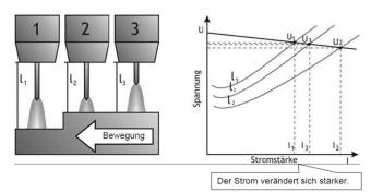
**Figure 1**: Interdependence of current, voltage and arc length for a flatly decreasing characteristic according to [1]
