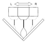
**Figure 3**: Different lengths of light arcs and the free rod end at different positions of the welding torch relative to the middle of the welding seam.
