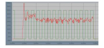
**Figure 10**: Recording of a voltage-controlled standard GMAW process. Image source: User
