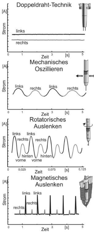
**Figure 4**: Scanning the groove with arc sensors according to DVS Information Sheet 0927-1 [1]
