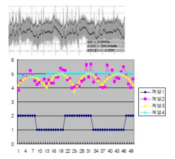
**Figure 11**: In spite of a turbulent noise process (grey presentation above), an auxiliary track correction signal (4th line, light-blue) could be derived from the filtered evaluation (3rd line, yellow) based on the seam tracking signal (2nd line, pink) and the time-shifted, synchronised oscillation signal (1st line, dark- blue). Image source: Hyundai Hi4 [3].
