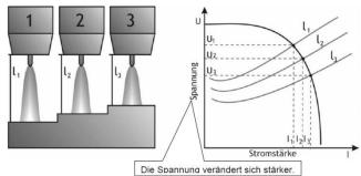
**Figure 2**: Interdependence of current, voltage and arc length for a strongly decreasing characteristic according to [1]
