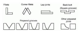
**Figure 7**: Recommended welding grooves for seam tracking, image source: FANUC [4]
