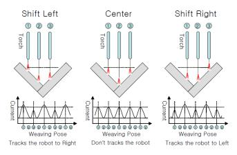
**Figure 5**: Principle of the evaluation of the "conventional" seam tracking signal for horizontal guidance, image source: Hyundai Hi4 [3]
