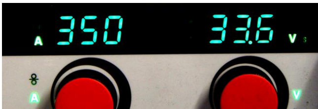
Figure 8: Setting the indirect welding current leading parameter (left button and display) and the desired average welding voltage (right button and display) using the Lorch MicorMig with Basic control panel.
