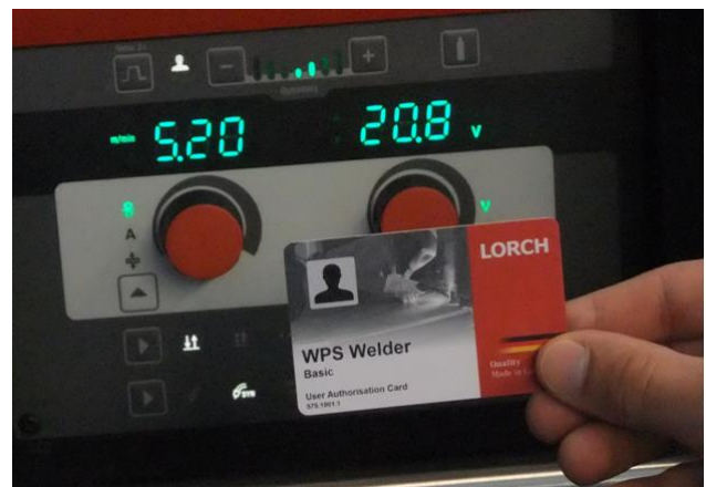
Figure 15: Realisation of a beneficial limitation of operating parameters through the user authorization concept.
