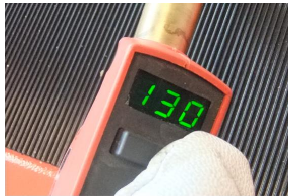
Figure 14: Adjusting the “dynamics” parameter at the torch. This is also possible during welding.
