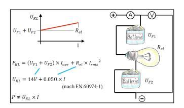
**Fig. 1**: Electrical equivocal circuit diagram for a simplified arc welding process model
