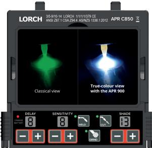
Operation and operating modes: Setting options for operating modes, protection level, delay, and sensitivity using clearly marked buttons with a display that can be read at any time. Welding mode (protection level 10-14), grinding mode (protection level 3), and cutting mode (protection level 5-9) are available in operation.
