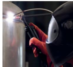
The **automatic cold wire feeder Lorch Feed** automates the manual feeding of filler material.
