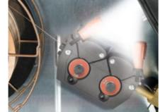
Interior lighting: For good visibility during wire threading in the easily accessible wire feed space with large robust flap.
