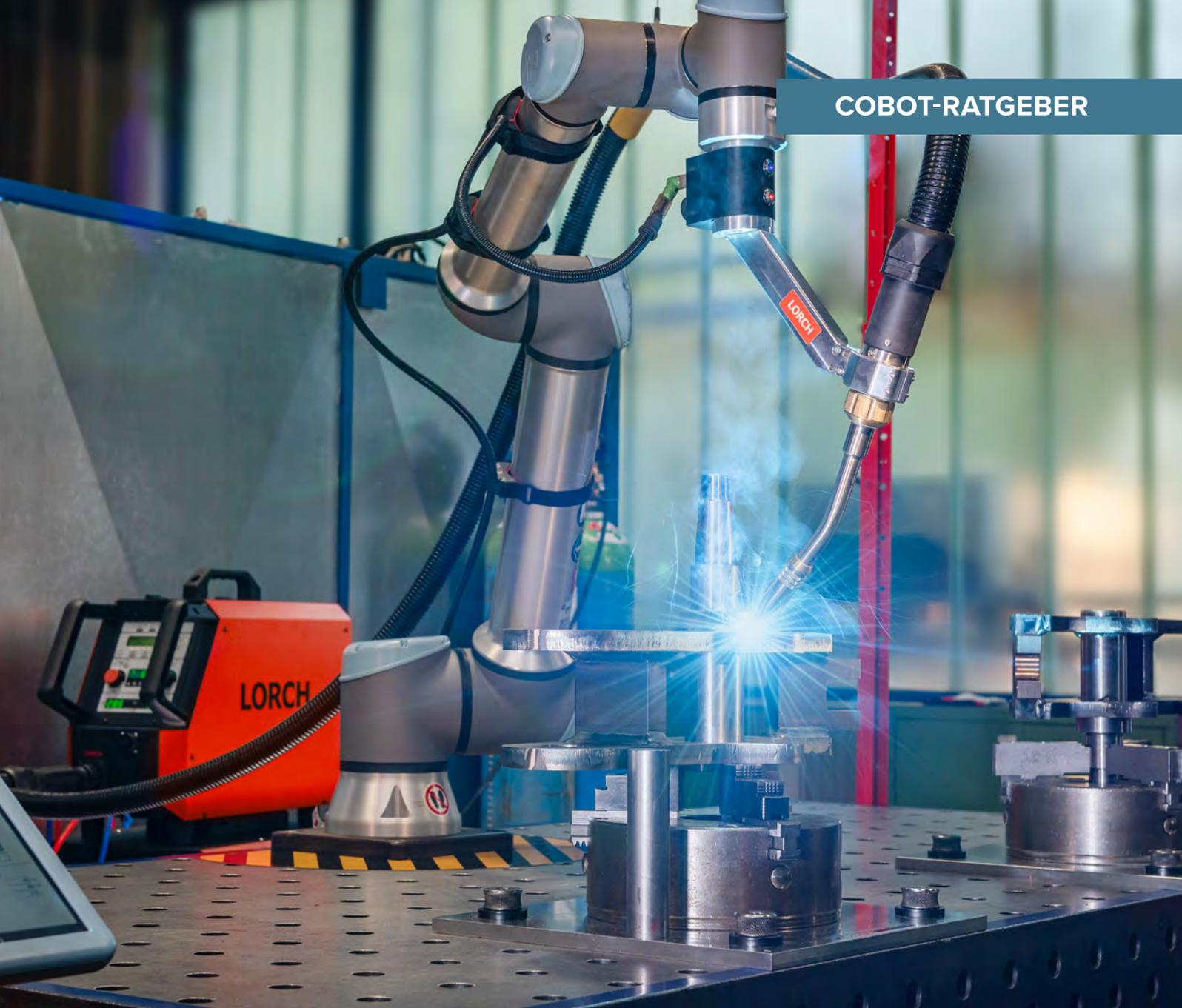
A close-up photograph of a silver robotic arm with a blue and red welding torch. The arm is positioned over a metal workpiece on a perforated metal table. A bright blue and white welding arc is visible at the point of contact. In the background, there is a blue safety enclosure and a red vertical beam. The overall scene is brightly lit, suggesting an industrial environment.
