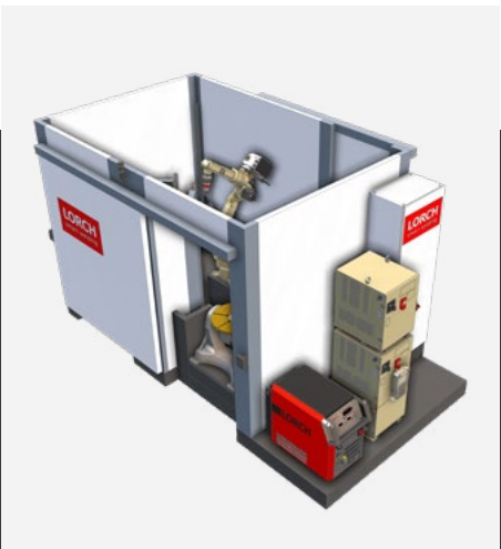
CUBE 05 2 x 2-axis turn/tilt positioner in different payload classes (300 and 500 kg).
