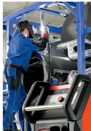
An end to unnecessary walking: Digital data coupling allows control of the most important welding parameters from the torch, even while the system is not in view. The figure shows the T300 AC/DC, which is optimised for industrial TIG production.
