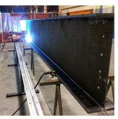
Quick and simple programming: The Trac RL Pro relieves weldersand ensures excellent longitudinal and curved welds.
