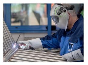
The energy input can be controlled with perfect precision with the T-Pro. This is extremely important when welding thin sheets.
