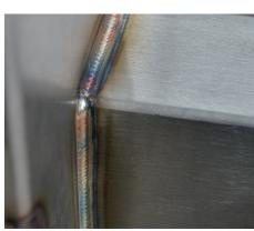
The best of weld seams: The weld seams must not have any depressions or pores in order to prevent the development of corrosion or microbes.
