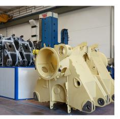
Thanks to the high strength of the Weldox special steel, parts like this chassis could be produced with a lower weight.
