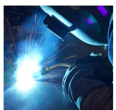
SpeedArc allows Mecalfast to not only weld the Weldox special steel more quickly now. The welding process also warrants precise and clean weld seams and little distortion.
