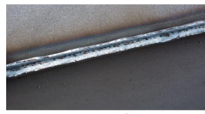
High-quality weld seam: The joints also visually offer an optimised weld appearance. Difficult areas such as tack welds and uneven gaps can be easily removed thanks to SpeedPulse XT. Just weld over it.
