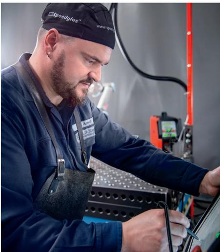
Simple operation: The welding process is "programmed" via the touch display. The torch may also be moved to the start and end positions manually via the free-drive function.
