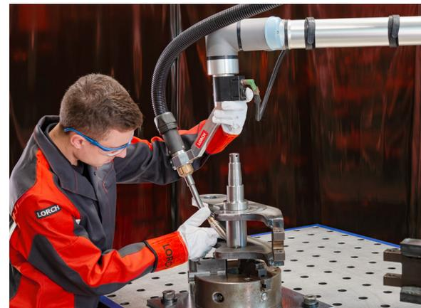
The innovative multifunctional flange and three freely assignable buttons permit direct integration of the practical additional Quick-Points feature for speedy teaching of parts on the Cobot.
