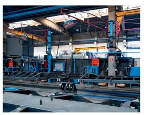
More than 160 MicorMIG 400 are working in the five plants of Faymonville Group. The MIG-MAG welding inverter scores with the SpeedArc process for a focused arc, high welding speed, and simple, multilingual operator guidance.
