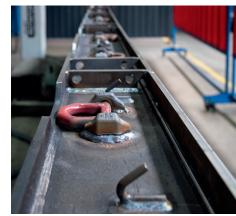
The MicorMIG plays all its strengths at Faymonville, with deep penetration, a lower number of layers, and a shorter welding time.
