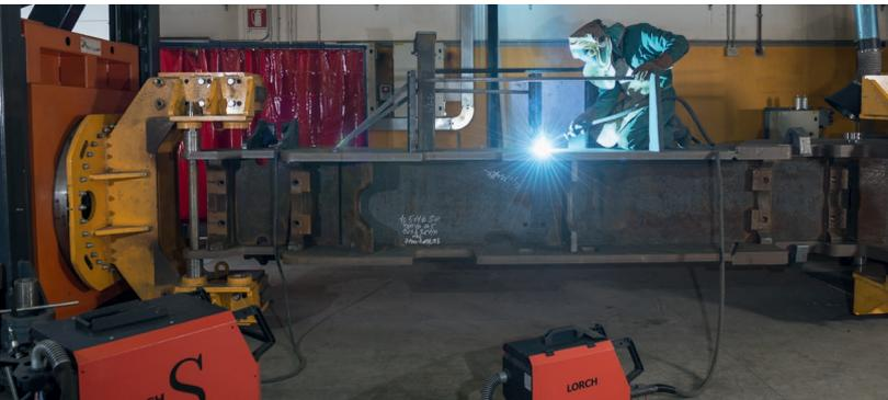
*"Compared to other suppliers' processes, the SpeedPulse process delivers a significantly higher welding speed with improved penetration at the same time. The stable arc gives us overall increased seam reliability at the same time."*
