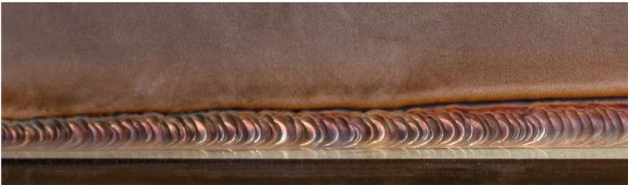
*Comparison: TIG with additional stainless steel fillet weld 6 mm*
