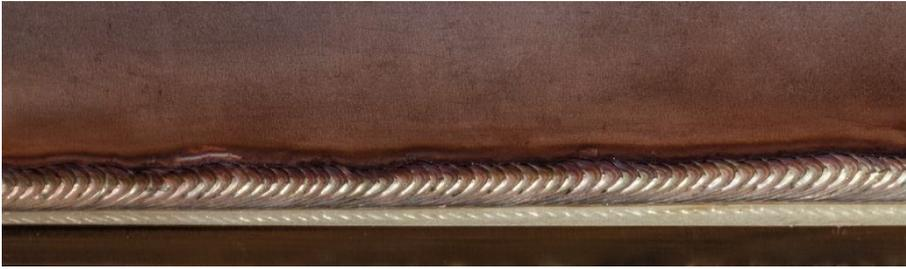
*MicorTwin stainless steel fillet weld 6 mm*
