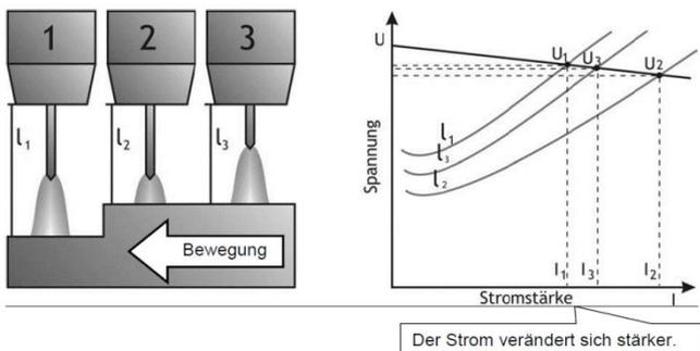
**Figure 1:** Interdependence of current, voltage and arc length for a flatly decreasing characteristic according to [1]
