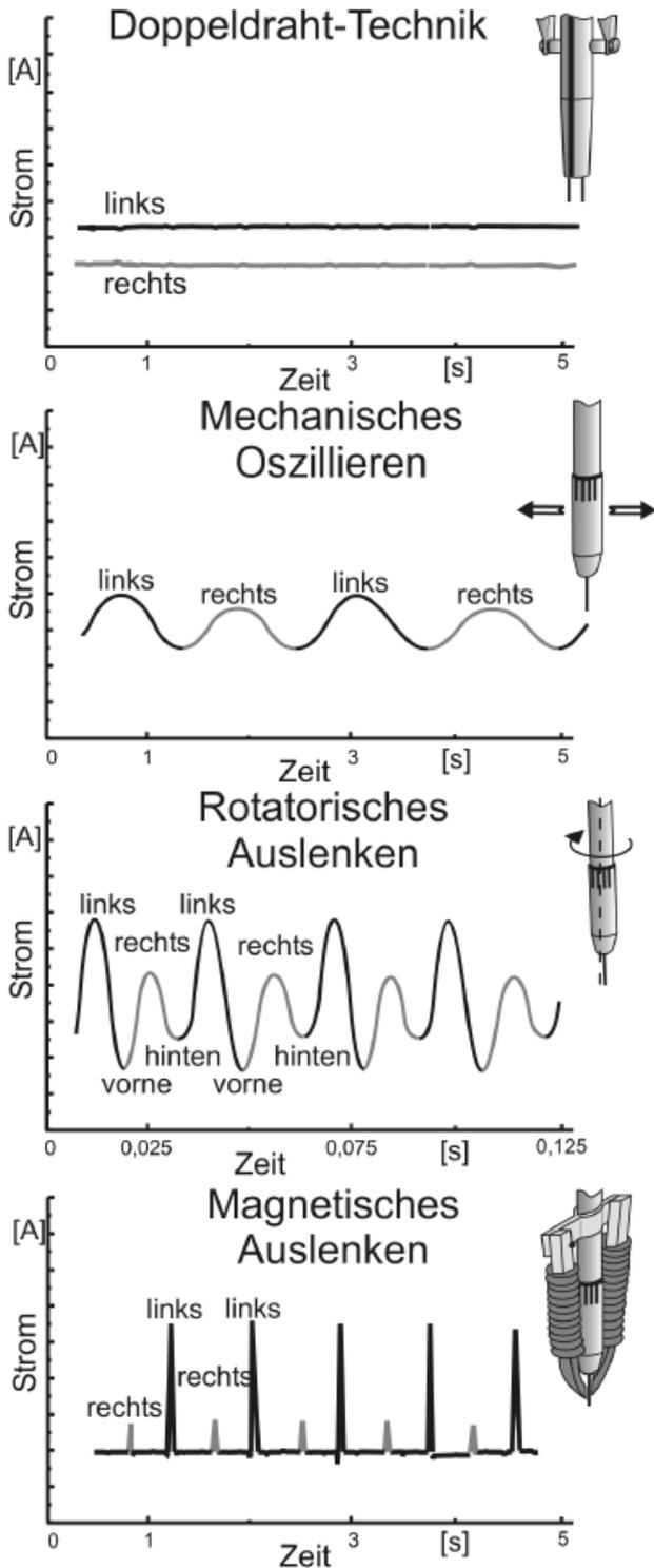
**Figure 4:** Scanning the groove with arc sensors according to DVS Information Sheet 0927-1 [1]
