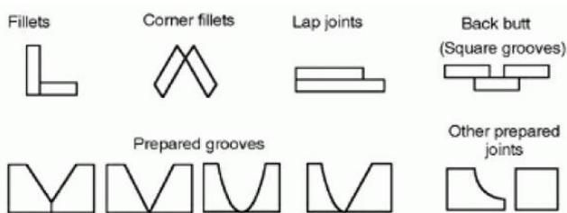
**Figure 7:** Recommended welding grooves for seam tracking, image source: FANUC [4]
