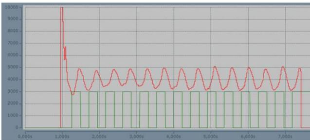
**Figure 9:** Recording of an oscillating, current-controlled impulse welding process on an angled sheet. Image source: User
