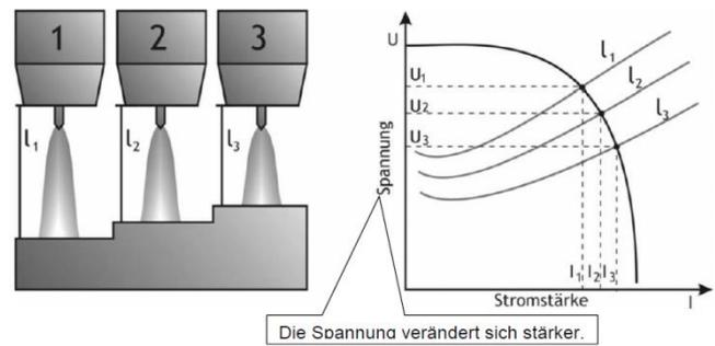
**Figure 2:** Interdependence of current, voltage and arc length for a strongly decreasing characteristic according to [1]
