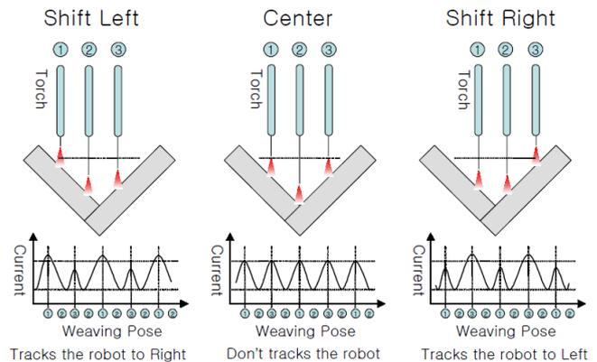
**Figure 5:** Principle of the evaluation of the "conventional" seam tracking signal for horizontal guidance, image source: Hyundai Hi4 [3]
