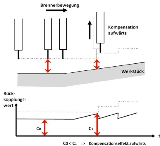
**Figure 6:** Principle of the evaluation of the "conventional" seam tracking signal for vertical guidance, image source: FANUC [4]
