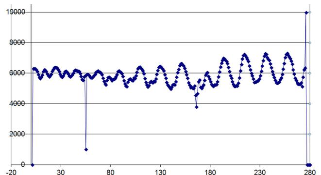
**Figure 8:** Presentation of a digitally recorded signal pattern of the seam tracking signal.
