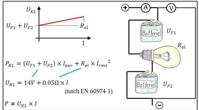
**Fig. 1:** Electrical equivalent circuit diagram for a simplified arc welding process model
