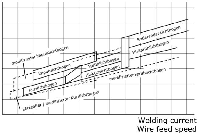
**Fig. 2:** General position of process windows and their expansions by modified process control variants
