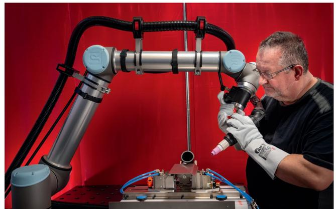
The free-drive function is very easily accessible for the welder right at the torch holder.
