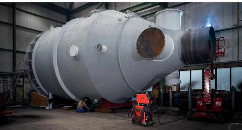
Far more than 1000 hours are required for welding an evaporator for the desalination plant. Weld seams must live up to the highest demands, and every single T-joint will be x-rayed individually.
