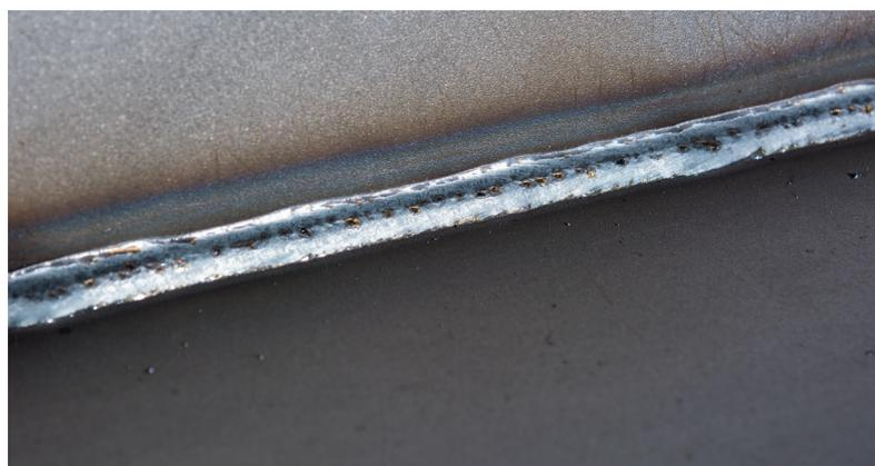
High-quality weld seam: The joints also visually offer an optimised weld appearance. Difficult areas such as tack welds and uneven gaps can be easily removed thanks to SpeedPulse XT. Just weld over it.
