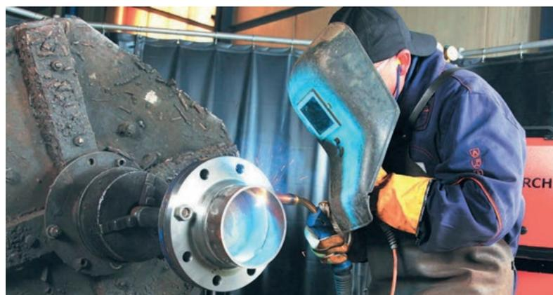
Luis Braga welds the root layer of the pipe socket with a Lorch S-SpeedPulse machine using Lorch's SpeedRoot process. The top layer is welded with Lorch SpeedPulse.
