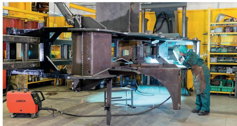
Ideal for large parts: The welding parameters can be set directly at the torch with the Powermaster remote control.
