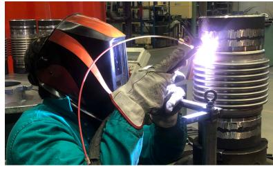
Precise weld seams and low material distortion enjoy the highest priority in production of the complex expansion elements (expansion vessels).
