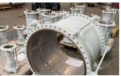
Indispensable in plant engineering: Expansion vessels compensate for the thermal and mechanical changes to the pipes. They need to be perfectly tight while remaining flexible. They can be as much as two metres in diameter.
